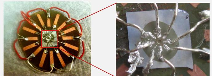
Board and electrical connections for actuation and sensing
