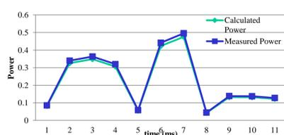
Comparison of measured and calculate TOTAL dynamic power over time
